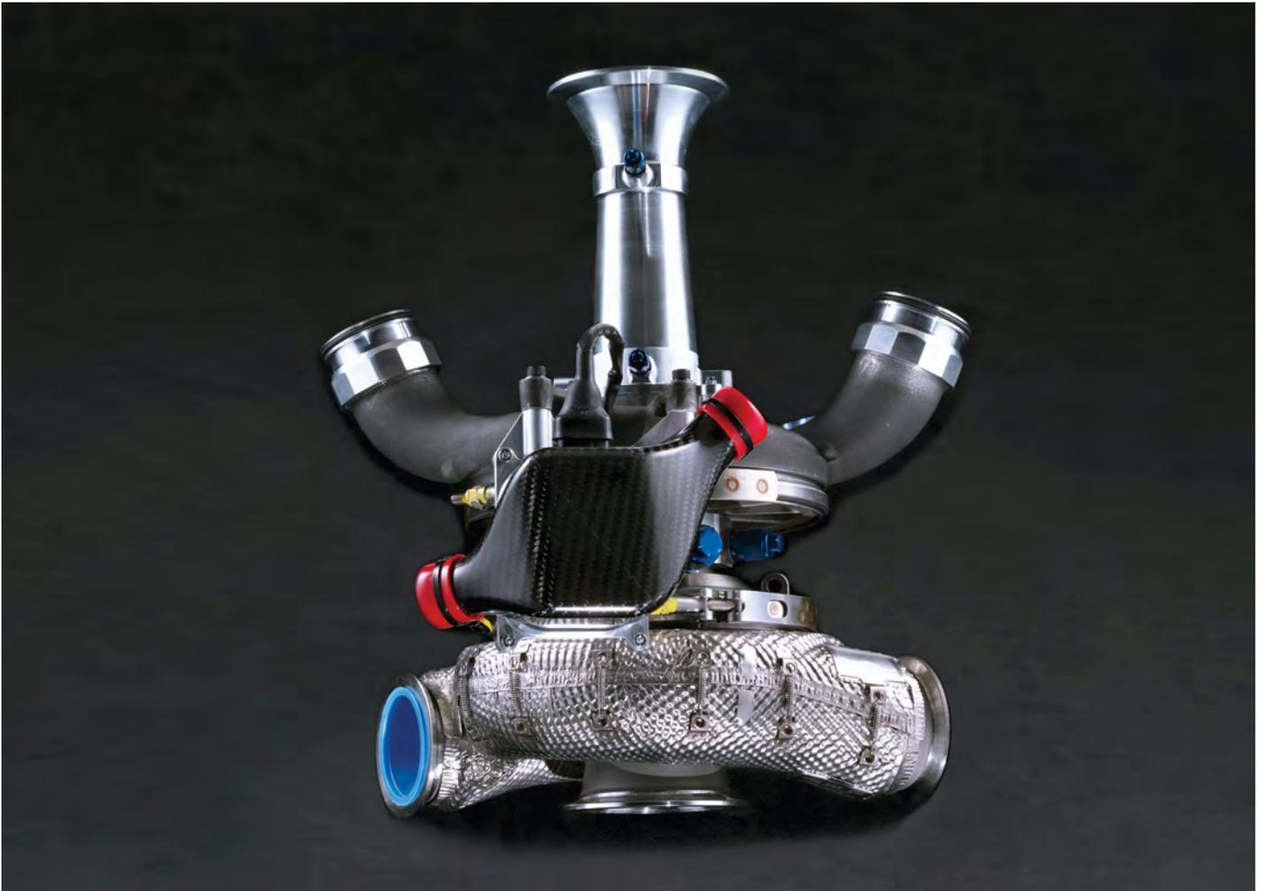
**Audi's VGT turbo was developed with Honeywell Turbo Technologies, and was used in both the R15 and R18 prototypes**
