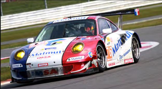
Powering the 911 GT3 RSR is a particularly efficient six-cylinder boxer engine with a four-litre capacity. With a mandatory air-restrictor, it generates 460 hp (338 kW) and drives the 310 millimetre wide rear wheels. The diameter of the front wheels has increased by 30 mm to measure 680 millimetres. The Porsche sequential six-speed gearbox is operated via paddle shifts on the steering wheel.
