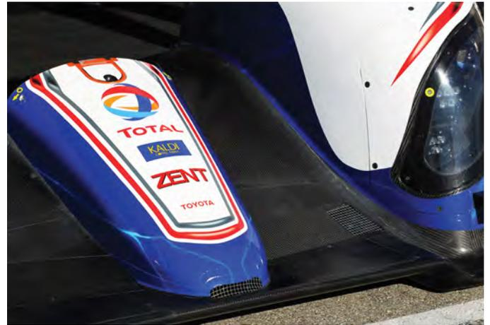
The new nose is lower than last year's model, meaning that Toyota will have to conduct new crash testing on the tub ahead of the first race in May
