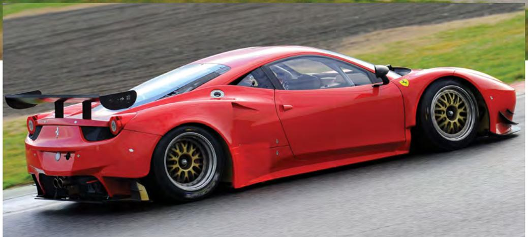
**The main update for the 458 is aerodynamic. The Ferrari has a wider front cross section compared to the Porsche, and has a lower top speed, which had to be increased without compromising fuel consumption**
