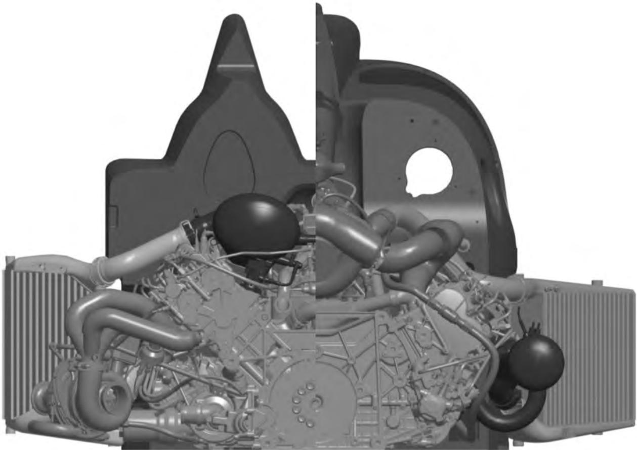
Side-by-side comparison of the engine bays of the R15 V10 TDI (left) and the R18 V6 TDI (right)
