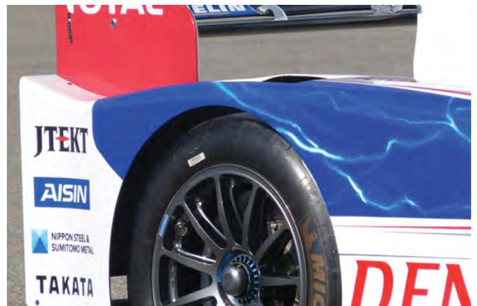
The TS030 was launched with the 2012 Le Mans bodywork. The team believes it can run its high downforce wheel arches at Le Mans
